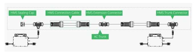
**Step 1** Connect the HMS Trunk Connector to the microinverter. Listen for a click as the connectors engage.
