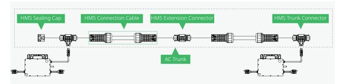
**Step 1** Connect the HMS Trunk Connector to the microinverter. Listen for a click as the connectors engage.
