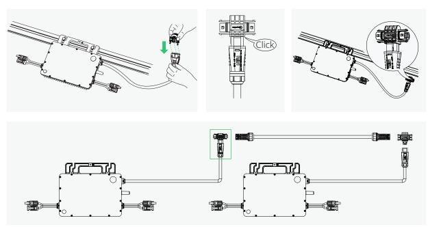
**Step 2** Cover the unused port on the HMS Trunk Connector (located at the beginning of the AC Trunk) with HMS Sealing Cap. Listen for a click as the sealing cap engages.
