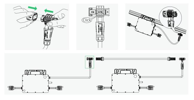
**Step 3** Use the HMS Connection Cable to connect the adjacent HMS Trunk Connectors. Listen for a click as they engage.
