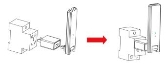
Option 2: Connect the DTU to the adapter and plug it into the Power Strip. Please make sure it is placed at least 0.5 meter above the ground and try to install the DTU
